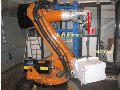
Figure 1. Experimental setup for the elastostatic calibration
